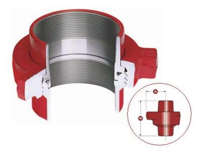
The suction and low pressure Figure 50 is manufactured from steel throughout and is available threaded or socket weld in 4" or 5" sizes. The same nut and 'O' ring are used in both sizes, male and female blanking caps are also available.
