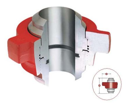
The 5" and 6" Fig. 1002 unions utilize elastomer "O" rings for sealing purposes. This type of union must be made up perfectly square and if not it can be troublesome. To improve matters, has introduced two new sizes of Butt Weld Unions that utilize lip type elastomer seals similar to those fitted into the smaller unions. These new sizes are referred to as "Fig. 1004".
