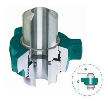
Standard service Fig. 2002 unions are manufactured throughout from the finest of steels selected to give the ultimate in performance. Lip type elastomer seals with anti-extrusion rings are supplied with this union. Available butt weld only.
